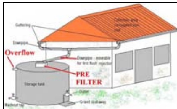
Figure 22: Basic principles of rainwater harvesting (Modified from the EU “DOMESTIC ROOFWATER HARVESTING IN THE HUMID TROPICS”).
