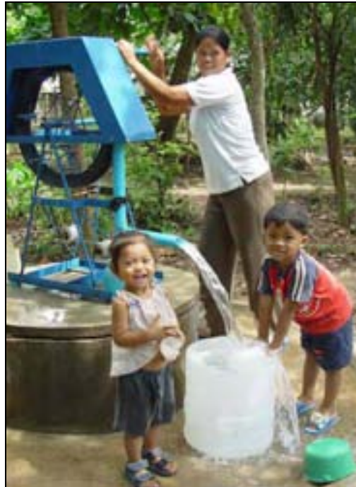
Figure 36: A rope pump installed in Cambodia.
