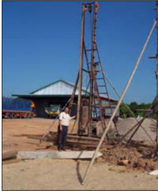
Figure 42: A simple “Free fall” winch observed in Banteay Meanchay which could easily be modified to be used for a bailer bucket in a well.
