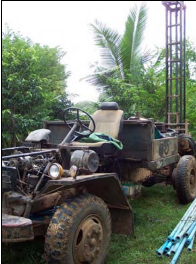
Figure 46: Details of a local small drilling rig.
